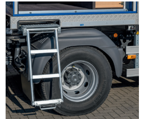
The box body can be conveniently loaded using the optional extendable ladder.
